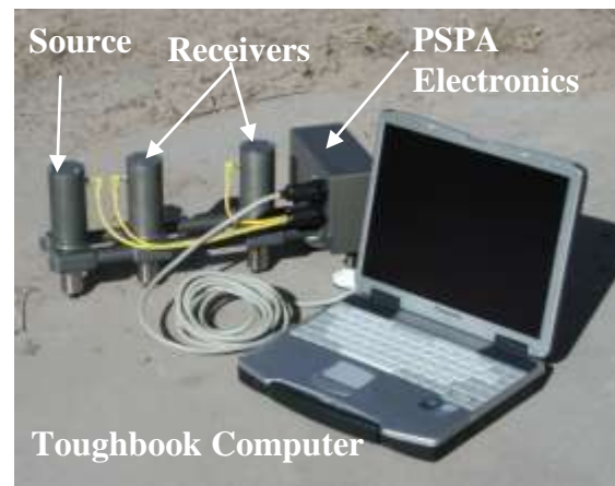
Figure 1. The PSPA System Components
